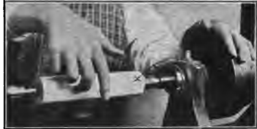
Fig. 10. Stopping the Lathe and Testing the Surface.
